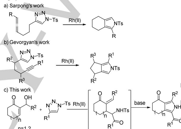
**Scheme 1** Rh (II) catalyzed reaction for the construction of 3,4-fused pyrroles.
