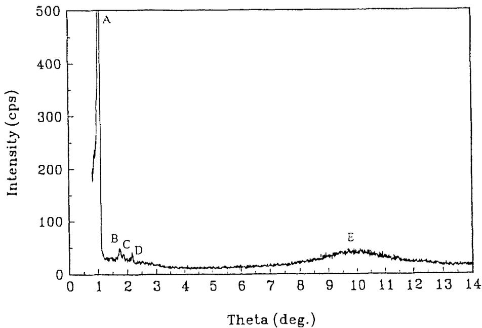
FIGURE 5 X-ray diffraction pattern of the columnar mesophase of compound 2 (95 °C)
