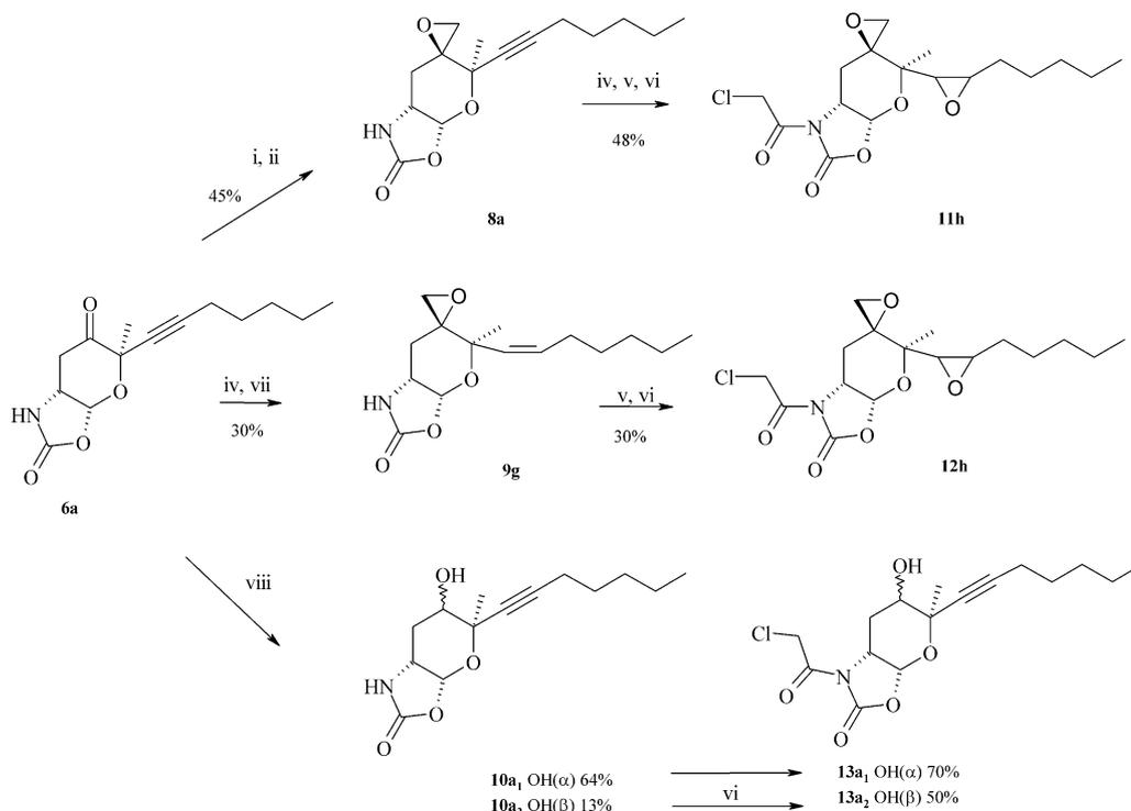
**Scheme 3.** Structural modifications at C<sub>1</sub>. (i) CH<sub>3</sub>PPh<sub>3</sub>Br, KOtBu, THF, 60 °C; (ii) MCPBA, CH<sub>2</sub>Cl<sub>2</sub>, rt; (iii) (a) nBuLi, THF, –78 °C; (b) ClCH<sub>2</sub>COCl; (iv) H<sub>2</sub>, Pd lindlar, C<sub>6</sub>H<sub>6</sub>; (v) 2,2-dimethyldioxirane, acetone; (vi) (a) nBuLi, THF, –78 °C; (b) ClCH<sub>2</sub>COCl; (vii) (CH<sub>3</sub>)<sub>3</sub>SI, nBuLi, rt; (viii) NaBH<sub>4</sub>, CeCl<sub>3</sub>, THF, –78 °C.
