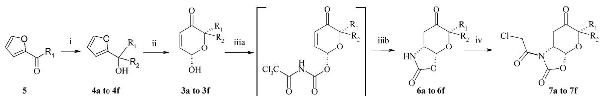
**Scheme 1.** Structural modification at C<sub>2</sub>. (i) R<sub>2</sub>Li, THF, -78 °C; (ii) NBS, THF, H<sub>2</sub>O, 0 °C; (iii) (a) CCl<sub>3</sub>CON=C=O, CH<sub>2</sub>Cl<sub>2</sub>; (b) NaHCO<sub>3</sub>, acetone; v: (a) *n*BuLi, THF, -78 °C; (b) ClCH<sub>2</sub>COCl.
