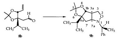
In a 50 mL round bottom flask were placed 300 mg (14.2 mmol) freshly chromatographed aldehyde **8b** and 290 mg (21.3 mmol) (S)- $\alpha$ -methylbenzyl hydroxylamine<sup>11</sup> in 30 mL reagent grade benzene. After stirring at reflux for 10h the solvent was removed at reduced pressure and chromatography of the resulting crude product (SiO<sub>2</sub>, 20% ethyl acetate/petroleum ether) yielded 256 mg (55%) of colorless isoxazolidine **9b**.
