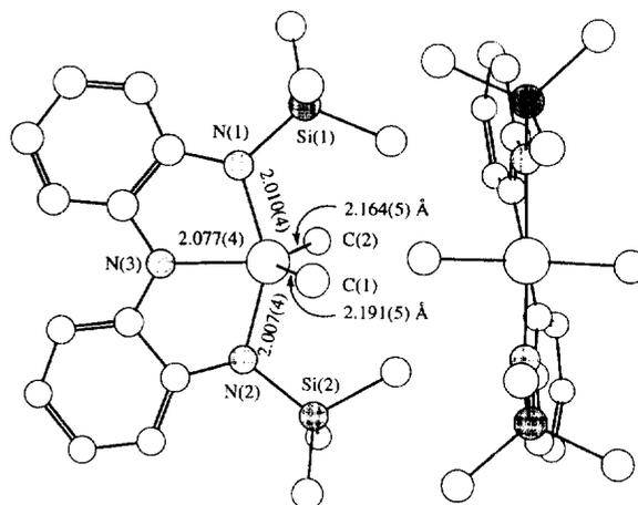
Fig. 1. Two views of the structure of  $[(\text{Me}_3\text{SiN}-o\text{-C}_6\text{H}_4)_2\text{N}]\text{TaMe}_2$ ; Ta–N(1)–Si(1) =  $117.2(2)^\circ$ , Ta–N(2)–Si(2) =  $115.8(2)^\circ$ . (See Table 2 for a comparison of bond lengths and angles in several structures.)
