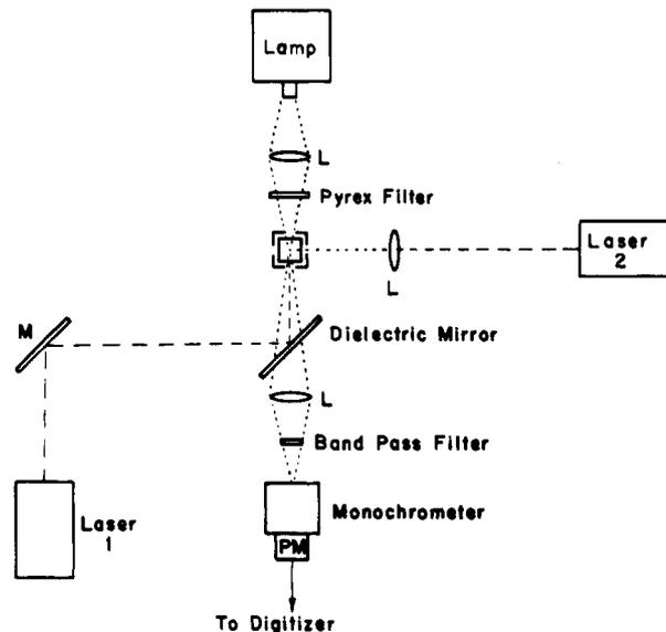
**Figure 2.** Photolysis arrangement used in these experiments. Laser 1 is at 248 nm and laser 2 at 355 nm or other wavelengths. The two mirrors for 248 nm have dielectric coatings and were optimized for 45° incidence. At the wavelength used for analysis the one mirror passes most of the analyzing light.
