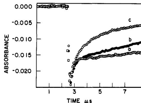
Figure 4. pH dependence of the bleach signal at 340 nm for 0.5 mM NaCl solution (total ionic strength 0.15 M): (a) pH 3.75, (b) pH 1.77, and (c) pH 1.20 (average of 25 shots each).
