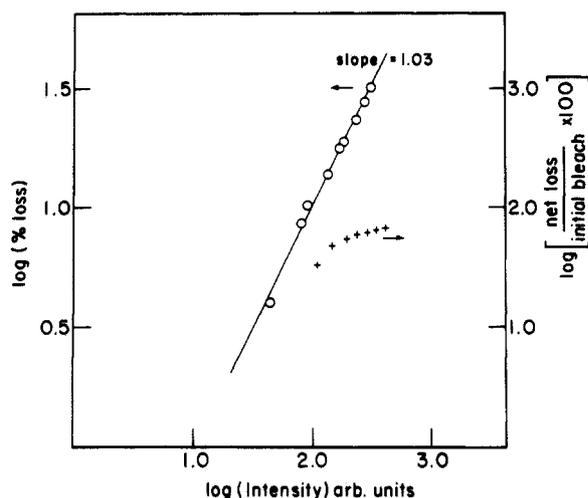
**Figure 5.** Intensity dependence of bleach and loss signals (see text). The bleach is defined as the initial amplitude immediately following the laser pulse, and the loss is the amplitude after the fast exponential recovery. (In Figure 4a the bleach is about 0.023 in absorbance and the loss is about 0.016.)
