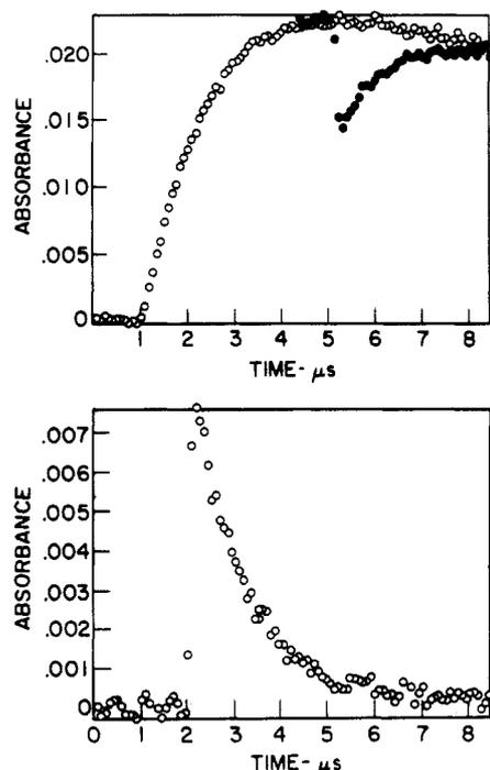
**Figure 3.** Top: Absorption profiles at 380 nm corresponding to 248-nm excitation alone (open circles) and to 248- and 355-nm excitation (closed circles) of 0.2 mM KI (average of 4 shots each). Bottom: The difference between the two signals above, obtained directly by the computer (as described in the text) and inverted for presentation, gives the bleach signal (15 shots). The digitizer was triggered at a later time so the time origin is offset.
