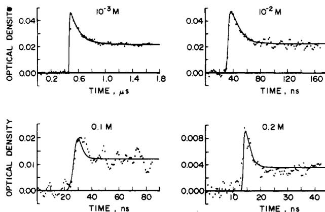
**Figure 6.** Experimental bleach signals (inverted) observed at 340 nm for 0.001 M (25 shots), 0.01 M (15 shots), and 0.1 M (50 shots) and at 360 nm for 0.2 M (50 shots) NaCl solutions. The first three sets are for 355-nm excitation, and that for 0.2 M is for 337-nm excitation with a 0.8-ns pulse. The calculated curves were obtained by numerically integrating the differential equations corresponding to the sequential reactions (8)–(10). The values of the parameters are given in the text.
