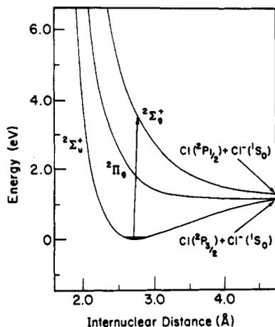
**Figure 1.** Potential energy curves for the ground and excited states of  $\text{Cl}_2^-$ —adopted from ref 5c and modified to include spin-orbit splitting of Cl. Only those excited states to which transition from the ground state is allowed are shown. The arrow indicates the transition corresponding to 355-nm excitation.
