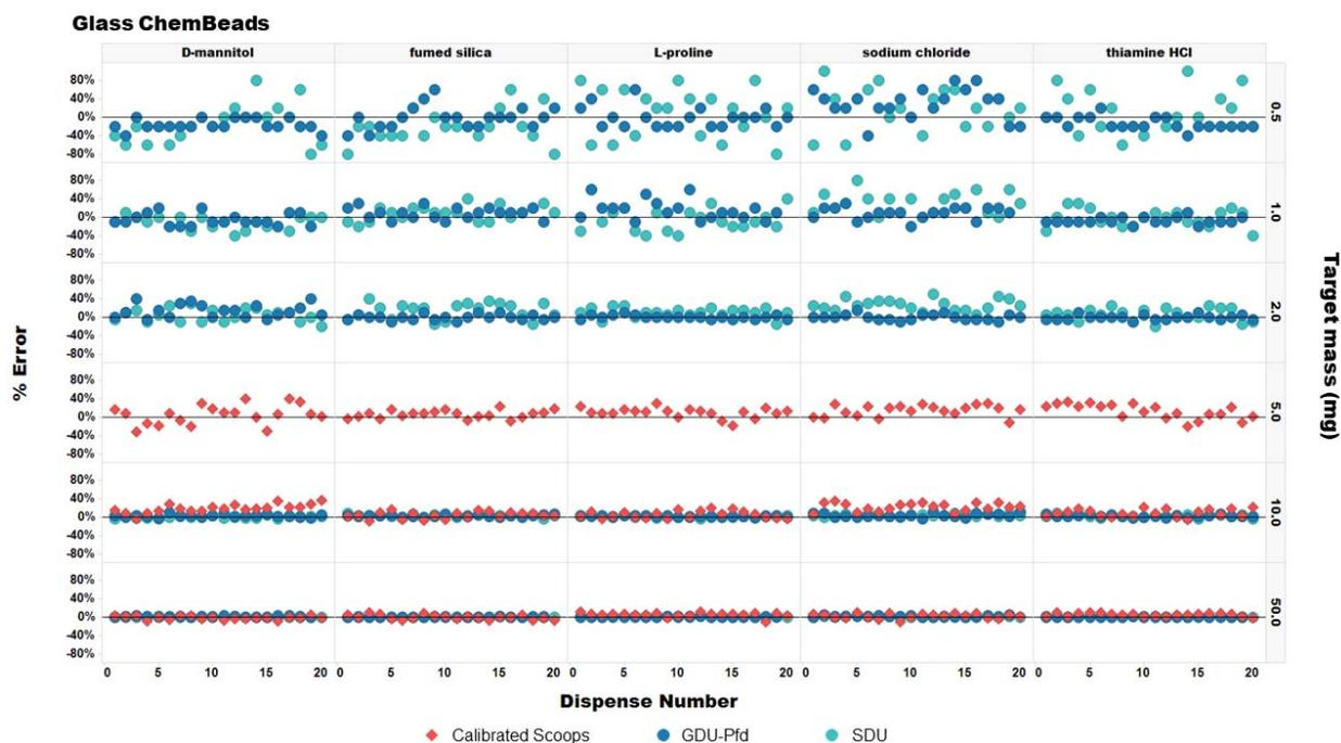
**Figure 1.** Scatterplot of % error values (-80% to 80%) vs. dispense number (1 – 20), broken down by reagents on glass beads (columns), target mass in mg (rows), and instrument (colors).
