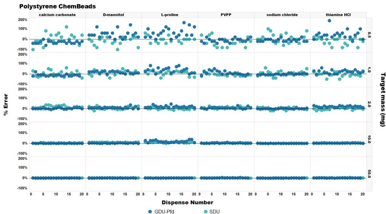
**Figure 2.** Scatterplot of % error values (-100% to 200%) vs. dispense number (1 – 20), broken down by reagents on polystyrene beads (columns), target mass in mg (rows), and instrument (colors).
