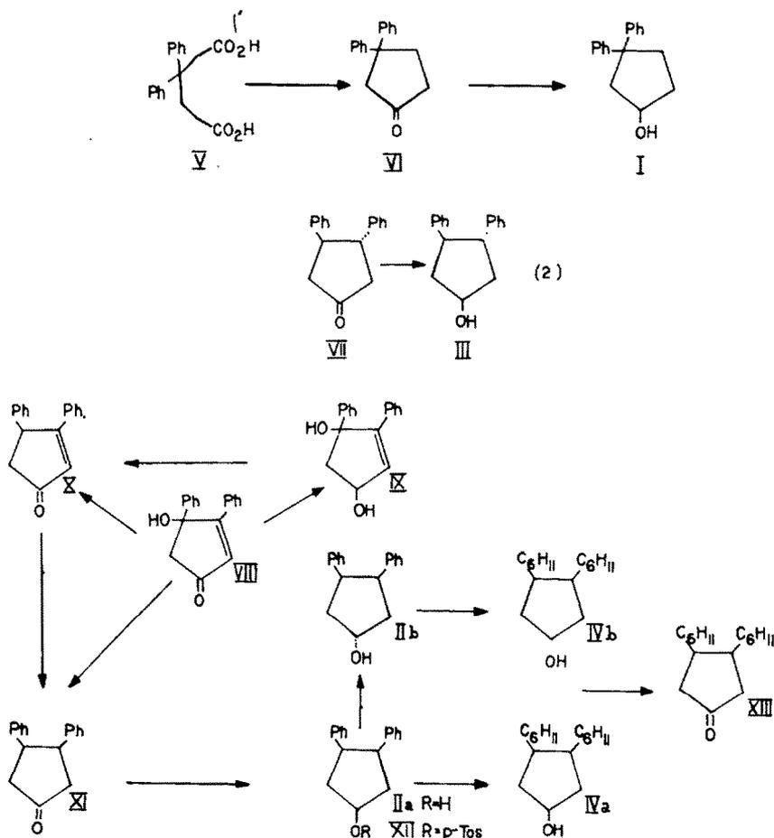
3,3-Diphenylcyclopentanol (I) (see Table 1 and subsequent discussion) was obtained by  $\text{LiAlH}_4$  reduction of the heretofore unknown ketone (VI). The latter was prepared by pyrolysing the Ba salt of 3,3-diphenyladipic acid<sup>3\*</sup> (see Table and subsequent discussion).
