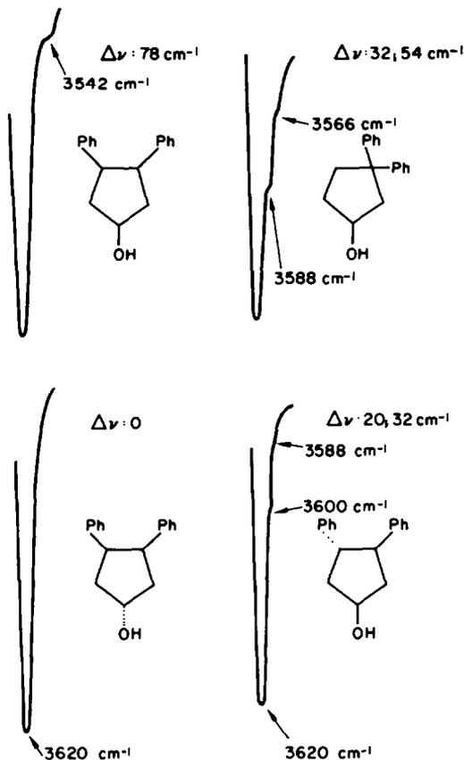
FIG. 1. IR absorption bands of dilute solutions of the alcohols in the  $3\mu$  range
