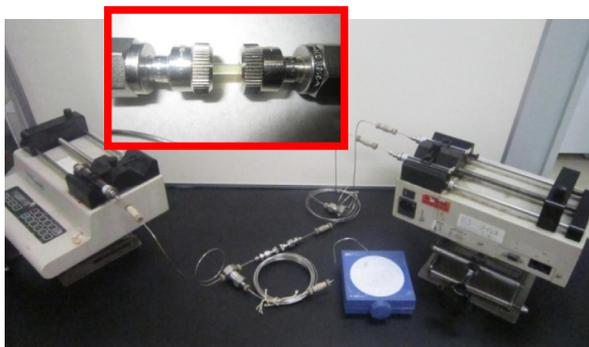
Figure 5. Flow microreactor system equipped with a quartz glass tube.
