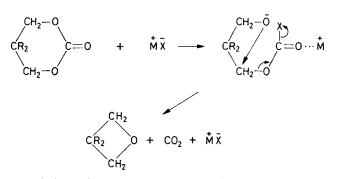
For the case of the polycarbonate, I, intramolecular reaction of the type indicated above would not be possible as too great a distortion of the normal valency angles would be required to produce a cyclic ether, so that the only ether which could be formed would be the polymeric structure, II.
