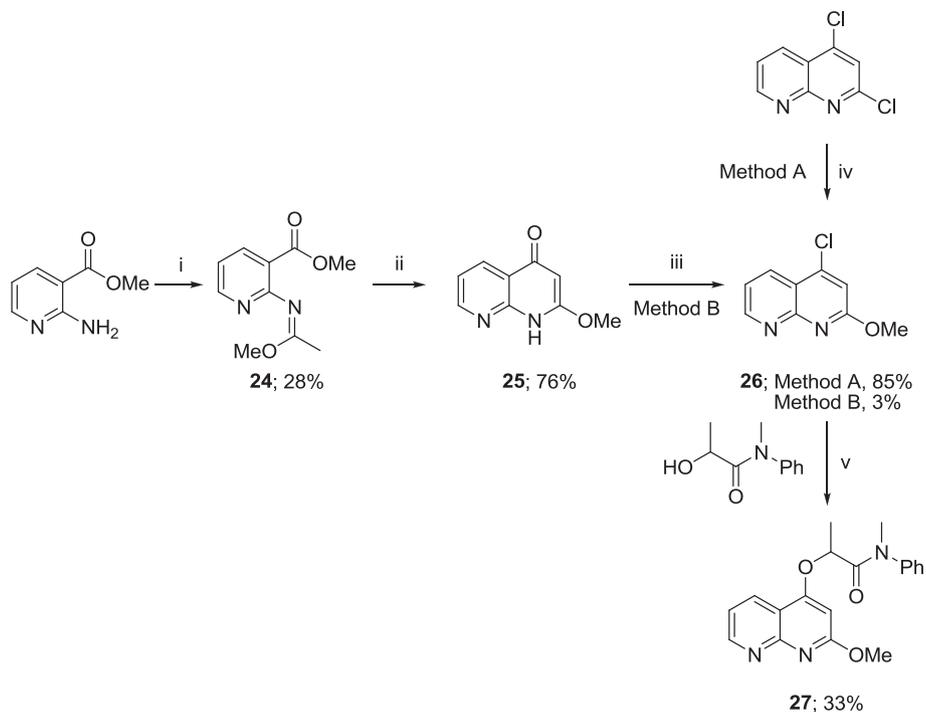
**Scheme 2.** Synthesis of the 2,4-dialkoxy-1,8-naphthyridine analog **27**. Reagents and conditions: (i) MeC(OMe)<sub>3</sub>, Ac<sub>2</sub>O, 110 °C; (ii) LDA, THF, hexane, –50 °C; (iii) POCl<sub>3</sub>, 110 °C; (iv) NaOMe, toluene, rt; (v) NaH, DMF, DMSO, rt.
