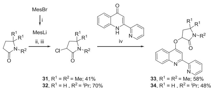
**Scheme 4.** Synthesis of  $\alpha$ -quinolinylolactam analogs **33** and **34** with eliminated amide bond rotation. Reagents and conditions: (i) *t*-BuLi, pentane, THF,  $-60$  to  $-70$  °C, then  $-20$  °C; (ii) THF,  $-70$  °C, then 0 °C; (iii)  $\text{C}_2\text{Cl}_6$ , THF,  $-78$  to  $-70$  °C, and then rt; (iv)  $\text{K}_2\text{CO}_3$ , MeCN, 80 °C.
