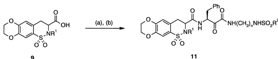
**Scheme 2.** Synthesis of compounds of Table 2. Reagents: (a)  $\text{HCl-H}_2\text{NCH(CH}_2\text{Ph)CH(OH)CONH(CH}_2\text{)}_n\text{NHSO}_2\text{R}^2$  (**10**), HOBt, BOP, NMM, DMF, rt; (b) Dess–Martin periodinane,  $\text{CH}_2\text{Cl}_2$ , *t*-BuOH, 0–20 °C, 1–24 h.
