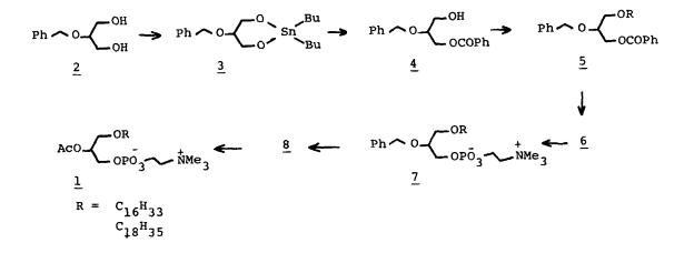
The preferred procedure involved treatment of 1 equivalent of the diol 2 $^6$  with 1 equivalent of di-n-butyl tin oxide in refluxing benzene for 6 hours to generate in quantitative yield the stannoxane 3 which was used without further purification. Compound 3 was then treated with one equivalent of benzoyl chloride in refluxing chloroform for 2 hours followed by the addition of one-third volumes of 4% aqueous dioxane. The homogeneous solution was refluxed
