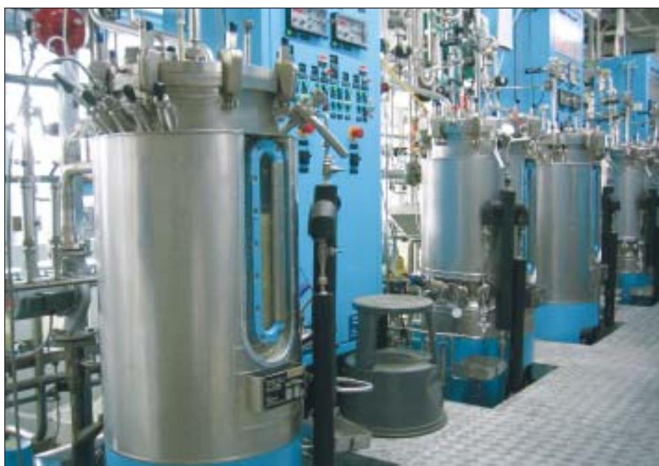
Fig. 1. Fermentor of 100 l used for the media preparation (Novartis AG)
