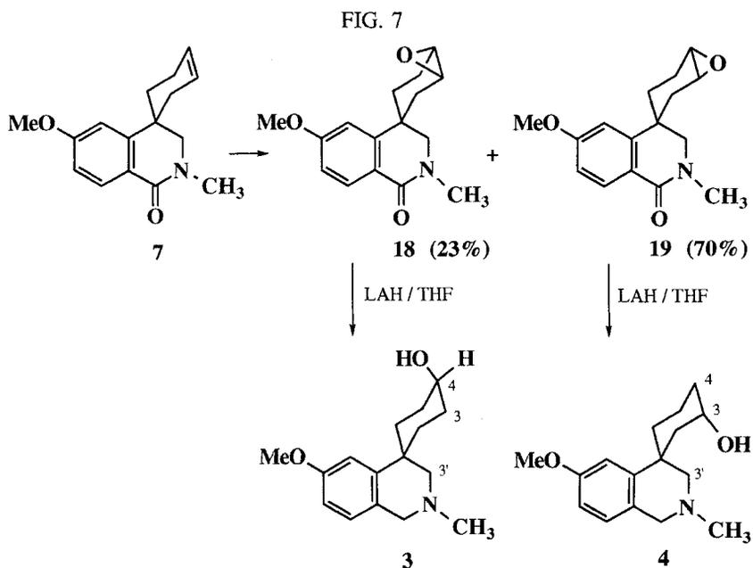
The two isomers could easily be separated by flash chromatography. The *exo* compound was the major product (7/3) and resulted from the attack of the reagent on the less hindered face of C ring, as shown by Molecular Modelling (figure 7).
