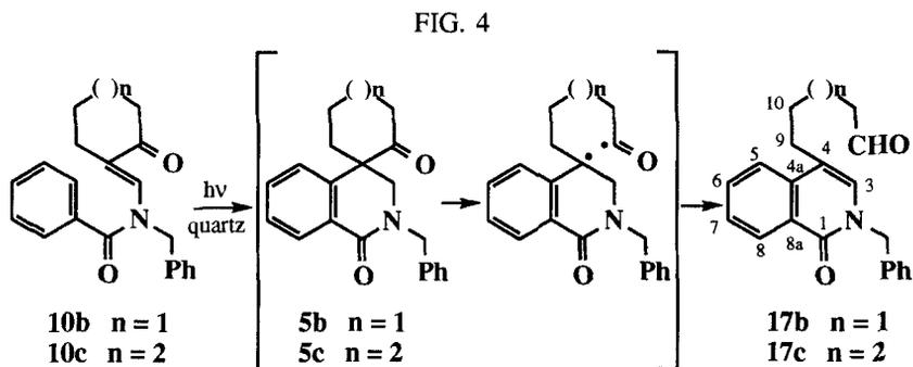
The use of a pyrex reactor with a cut off wavelength of 300 nm avoids the Norrish 1 cleavage and spiroketones **5** are thus obtained in good yields (figure 5).
