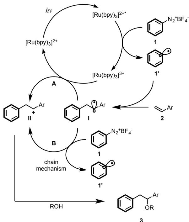
**Scheme 3.** Plausible reaction mechanism; (A) photo catalytic mechanism. (B) radical chain mechanism.
