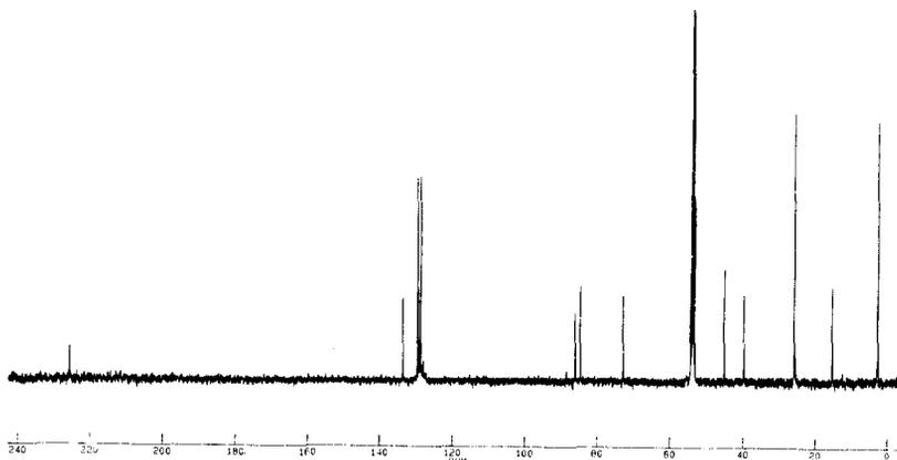
Fig. 3.  $^{13}\text{C}$  NMR spectrum of **9** at  $-70^\circ\text{C}$  ( $\text{CD}_2\text{Cl}_2$ )
