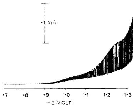
**Figure 1.** Dc polarogram: PAR 174 instrument with conventional dropping mercury electrode; concentration of malonaldehyde =  $1.5 \times 10^{-2}$  M in 2 M HCl; drop time = 0.5 s.
