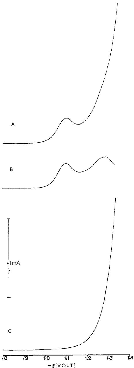
**Figure 2.** Differential pulse polarogram: PAR 374 instrument with 303 static mercury drop electrode; drop time = 0.5 s; concentration of malonaldehyde =  $9 \times 10^{-4}$  M in 2 M HCl; (A) without blank subtraction; (B) with blank subtraction; (C) blank.
