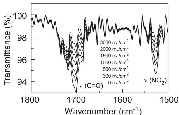
**FIGURE 3** IR absorption spectra of the PNC2-4 ( $M_w = 56,000$ ) film spin-coated on a KBr plate. Film thickness was 2  $\mu$ m. Sample film was irradiated at 254 nm.
