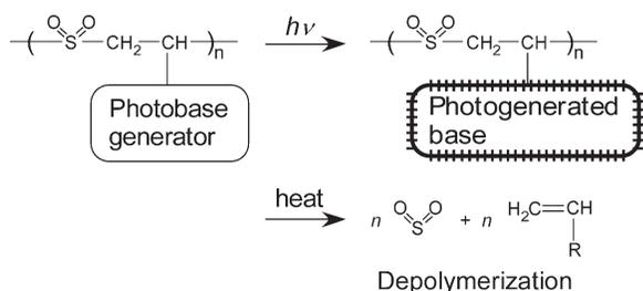
**FIGURE 1** Photoinduced depolymerization of poly(olefin sulfone)s possessing a photobase generator in the side-chain.
