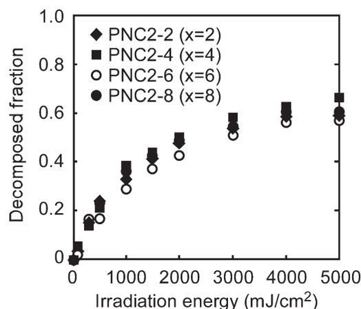
**FIGURE 4** Dependence of the photochemical reaction of the photobase generator in PNC2- $x$  film on irradiation energy. UV Light (254 nm) from a super-high-pressure mercury lamp was used to irradiate the film. Molecular weights ( $M_w$ ) of the polymers were 87,000 for PNC2-2, 56,000 for PNC2-4, 96,000 for PNC2-6, and 80,000 for PNC2-8.
