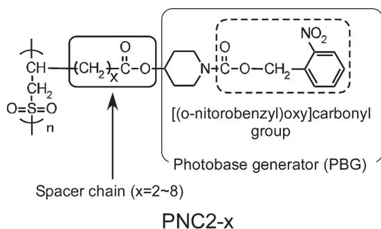
**FIGURE 2** Structure of poly(olefin sulfone)s PNC2-x ( $x = 2-8$ ).
