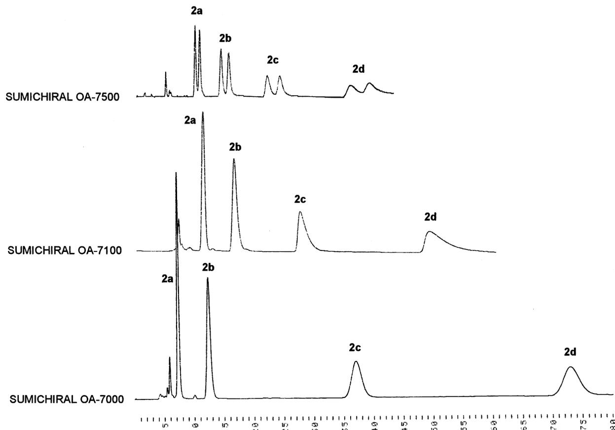
**Figure 2.** HPLC chromatograms of racemic alcohols **2a–d**. Top: CH<sub>3</sub>CN/H<sub>2</sub>O=55/45, 0.5 mL/min, 254 nm UV. Middle and bottom: 0 to 60 min, CH<sub>3</sub>CN/H<sub>2</sub>O=60/40 up to CH<sub>3</sub>CN/H<sub>2</sub>O=80/20; 60 to 80 min, CH<sub>3</sub>CN/H<sub>2</sub>O=80/20, 0.5 mL/min, 254 nm UV.
