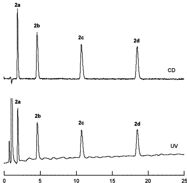
**Figure 1.** HPLC chromatograms of alcohols **2a–d**. Column: Fluofix 120E; mobile phase:  $\text{CH}_3\text{OH}-\text{H}_2\text{O}$  (0 to 30 min, 80/20 up to 100/0 v/v); flow rate: 1.0 mL/min; detector: 268 nm CD and UV.
