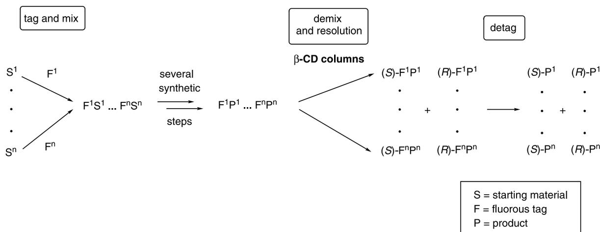
**Scheme 1.** Enantiomeric resolution of fluororous mixture by chiral  $\beta$ -CD columns.
