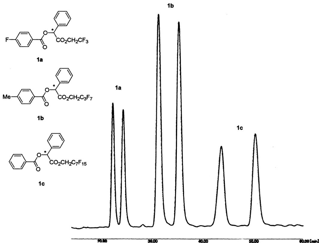
**Scheme 2.** Resolution of *O*-benzoylmandelate derivatives **1a–c** with β-CD column. Column: OA-7500: mobile phase, methanol–water (0 to 60 min, 75/25 up to 85/15, v/v); flow rate, 0.5 mL/min; detector, absorption at 254 nm; column temperature, 20°C.
