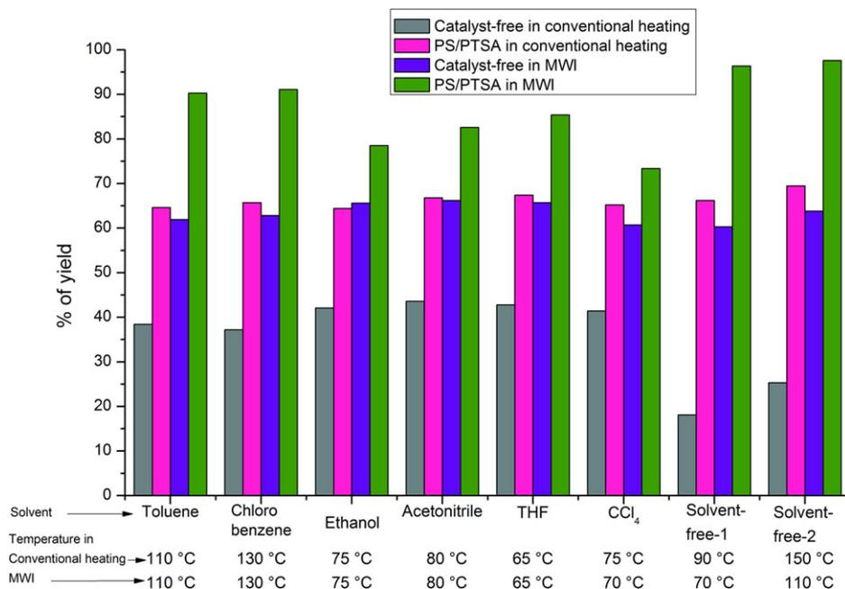
FIGURE 1 Optimization of solvent and temperature for the synthesis of **4a-r** in both conventional heating and MWI.
