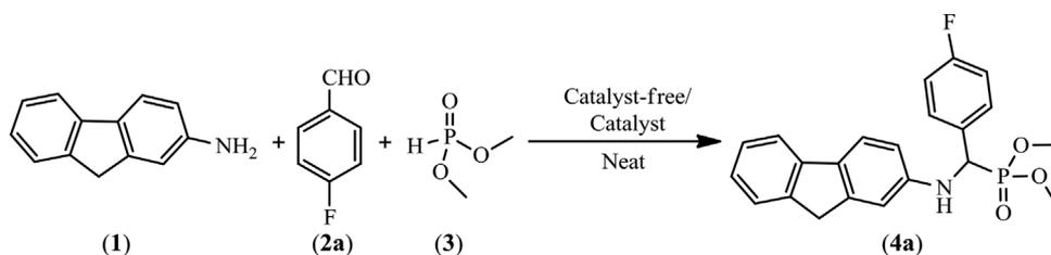
Reaction conditions: a) Conventional method, 70–120 °C, 55–140 min; b)  $\mu$ W method, 70–120 °C, 5–10 min
