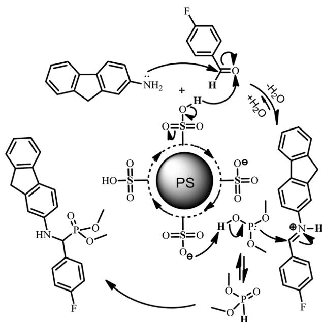
**SCHEME 3** Mechanistic pathway for one-pot KF synthesis of **4a–r** with PS/PTSA as a catalyst.
