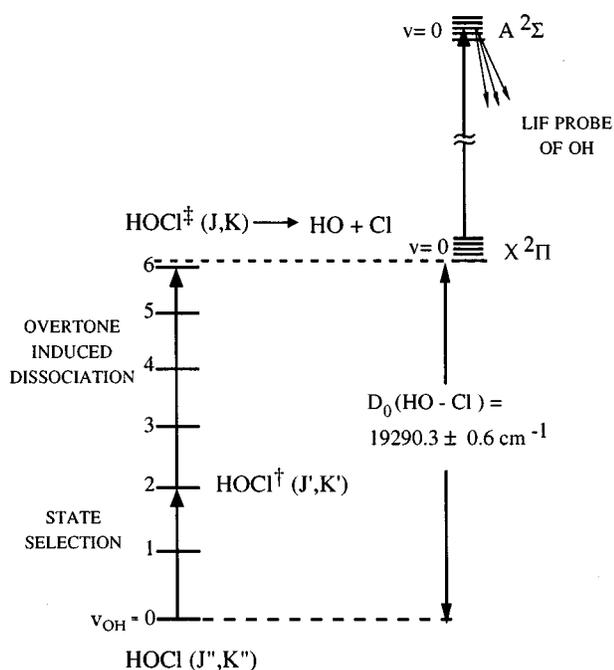
FIG. 1. Energy level schematic for  $2 \leftarrow 0$ ,  $6 \leftarrow 2$  double-resonance overtone excitation used to access single rovibrational eigenstates in the  $6\nu_1$  band of HOCl.
