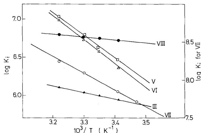
Fig. 2. Van't Hoff plots of PPxy-derivatives. (○—○) PPxy-L-tyrosine; (●—●) PPxy-D-tyrosine; (△—△) PPxy-L-tryptophan; (□—□) PPxy-L-phenylalanine; (▲—▲) PPxy-tyramine. The values of  $\log K_i$  for PPxy-L-tyrosine are shown at the right side of the graph, all the others at the left side
