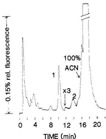
**Figure 5.** Separation of a derivatized bourbon sample, with fluorescent detection. Acrolein and crotonaldehyde peaks are as follows: (1) benzanthrone and (2) 1-methylbenzanthrone. Sensitivity of the fluorometer increased by 3 at 12 min. Mobile phase as in Figure 4 until switched to 100% acetonitrile at 15.8 min.
