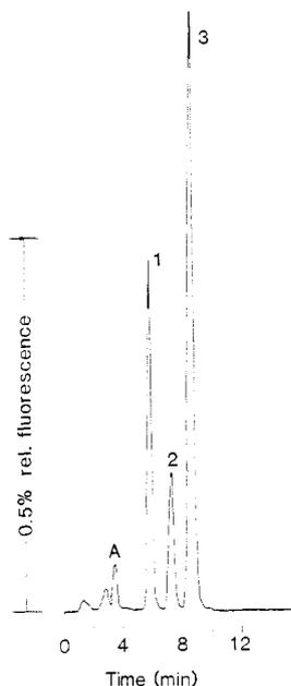
**Figure 3.** Fluorescent detection of an anthrone derivatized mixture of three vinyl aldehydes acrolein, crotonaldehyde, and methacrolein, all at approximately 9 ppm in 50% ethanol. The respective products are (1) benzanthrone, (2) 1-methylbenzanthrone, and (3) 2-methylbenzanthrone. The anthrone reagent peak is indicated by A. The mobile phase of 60/40 acetonitrile–water was pumped at 2.5 mL/min.
