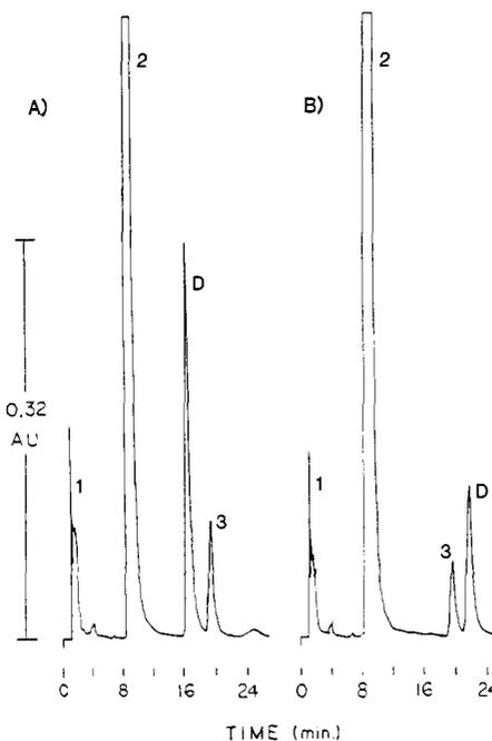
**Figure 2.** UV detection of anthrone derivatized (A) 22.2 ppm acrolein and (B) 21.5 ppm crotonaldehyde in water with respective products benzanthrone and 1-methylbenzanthrone labeled D. Other major peaks are as follows: (1) sulfuric acid, (2) anthrone, and (3) dianthrone. The mobile phase of 52/48 acetonitrile–water was pumped at 2.0 mL/min.
