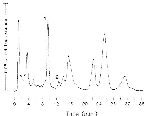
**Figure 4.** Separation of a derivatized Scotch whiskey (brand X) sample, with fluorescent detection. Acrolein and crotonaldehyde peaks are as follows: (1) benzanthrone and (2) 1-methylbenzanthrone. The mobile phase of 45/10/45 acetonitrile–methanol–water was pumped at 2.7 mL/min.
