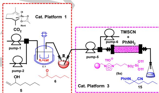
**Figure 9.** Schematic representation of the reactor set-up combining catalytic platforms 1 and 3 for the conversion of **5** into **15** catalysed by **Ru-4** and **9a**.
