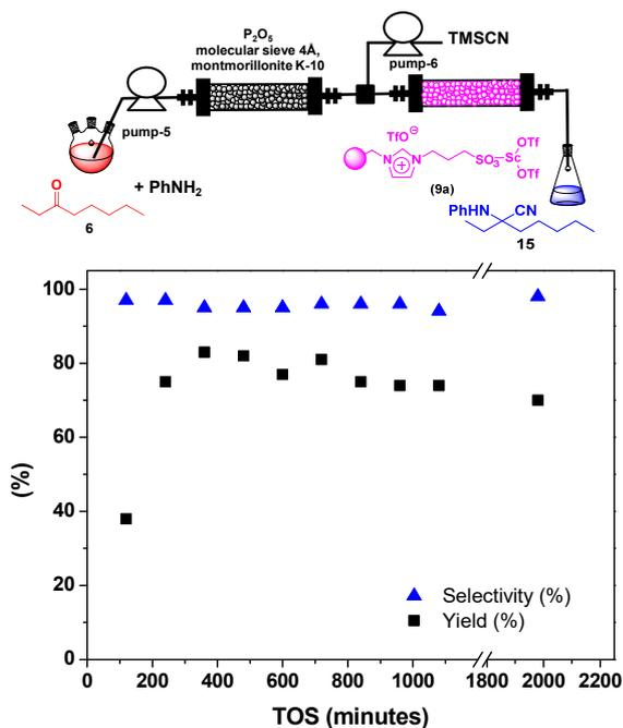
**Figure 11.** Yield and selectivity for **15** vs. time on stream (TOS) for the Strecker reaction of ketone **6**, aniline (**12**) and TMSCN catalysed by **9a** and set-up used for the reaction. Reactor I: 1.2 g of 4Å molecular sieves, 1.2 g  $P_2O_5$  and 1.2 g of MMK10, 3.9 mL reactor volume. Reactor II: 0.6 g of catalyst **9a**, 1.9 mL reactor volume.
