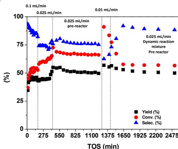
**Figure 10.** Results obtained combining the catalytic platforms 1 and 3. Conversion, yield and selectivity of **15** vs. time on stream (TOS) for the Strecker reaction of ketone **6**, aniline (**12**) and TMSCN catalysed by **9a**. 0.6 g of catalyst **9a**, 1.9 mL reactor volume.
