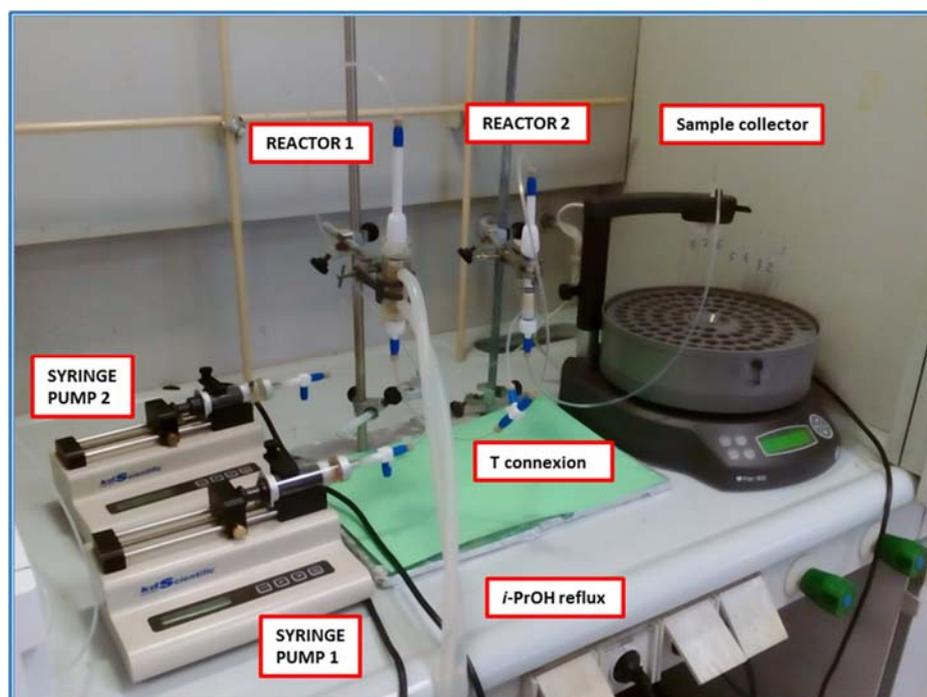
The second strategy used in order to push further the formation of the selectivity limiting ketamine, was to build a previous dehydrating catalytic reactor to favour the formation of the imine (see Figure S8).
