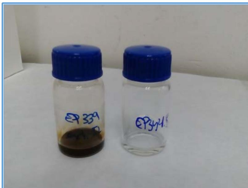
Figure S1.  $\text{Et}_2\text{O}$  (left) vs  $\text{scCO}_2$  (right) extraction of the 3-octanone (**6**)
