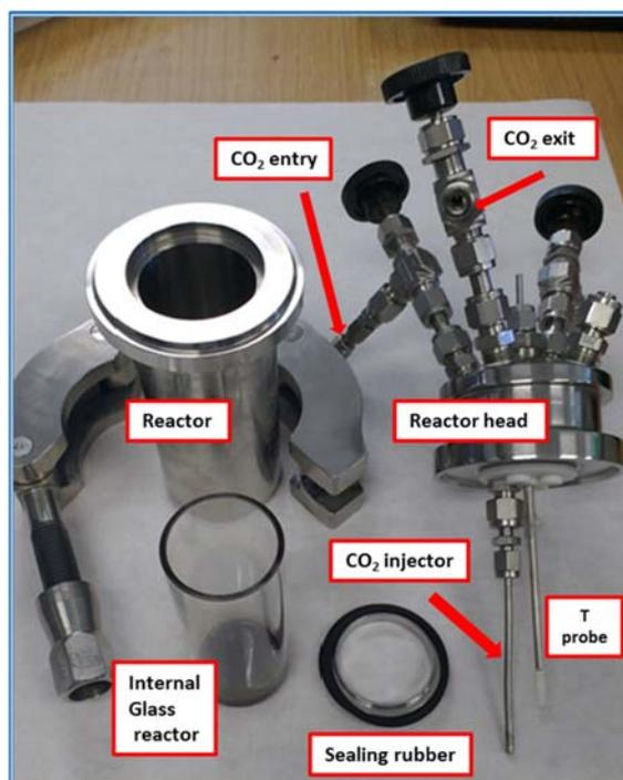
Figure S4. Parts of the pressure reactor used
