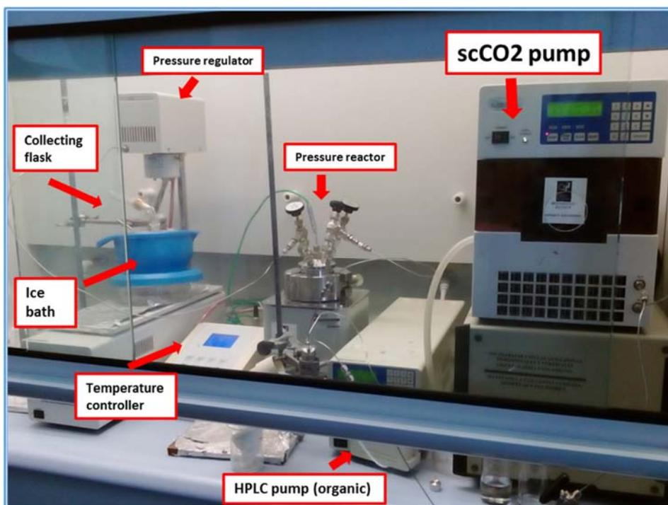
Figure S3. Set-up used for the continuous flow isomerisation of 1-octen-3-ol (5) into 3-octanone (6) using scCO<sub>2</sub>
