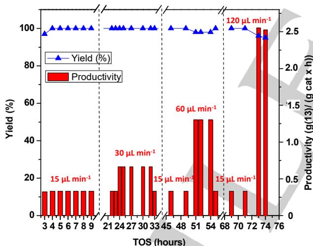
**Figure 8.** Yield of **13** vs. time on stream (TOS) for the three-component Strecker reaction of benzaldehyde (**10**), aniline (**12**) and TMSCN catalysed by **9a** under continuous flow. 1.5 M in 2-Me-THF, 0.850 g of catalyst **9a**, 2.4 mL reactor volume.
