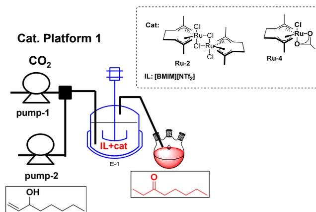
**Figure 2.** Schematic representation of the IL/scCO<sub>2</sub> set-up used for the isomerisation of **5** catalysed by **Ru-2** and **Ru-4**.
