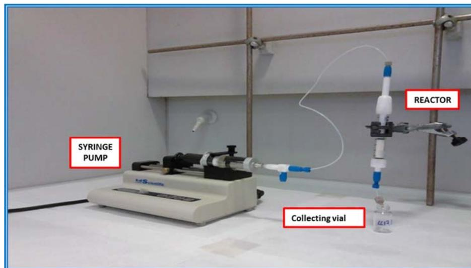
**Figure S6.** Set-up used for the continuous flow Strecker reaction of benzaldehyde (**10**). Syringe pump from kdScientific and Hamilton 25 mL syringe were used. Glass Omnifit column 006RG-10-10 (0.7854 cm diameter x 10 cm length) was used as reactor. The syringe was filled with a mixture of benzaldehyde (**10**), aniline (**12**) and TMSCN (1:1:1.2) 1.5 M in 2-MeTHF. The reactor was packed with 850 mg of SILLP-**9a**. The samples were collected in 12 mL glass vials.
