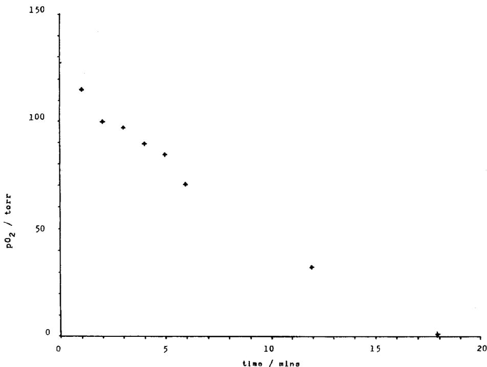
Fig. 14.  $p(\text{O}_2)$  during gas separation experiment.
