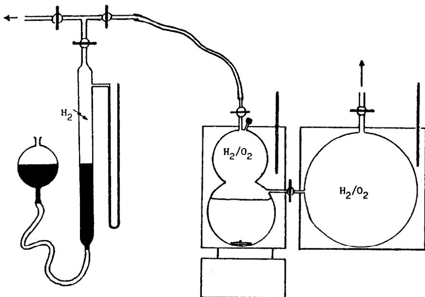
Fig. 12. Apparatus for separation of gas mixtures:  $H_2/O_2$  separation shown.
