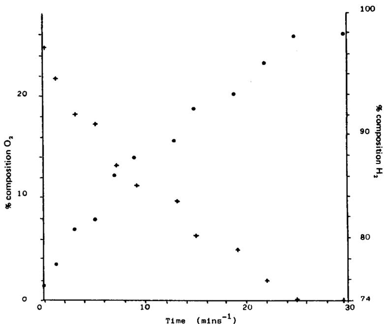
Fig. 16. Percent H<sub>2</sub> and CO during the gas separation experiment. ● = % H<sub>2</sub>, + = % CO.
