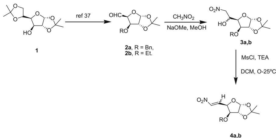
**Scheme 1.** Synthesis of nitrovinyl glucofuranose.
