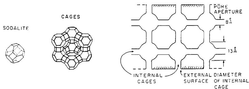
Figure 1. Representations of the building blocks, structure, and simple topological picture of the faujasite zeolite.
