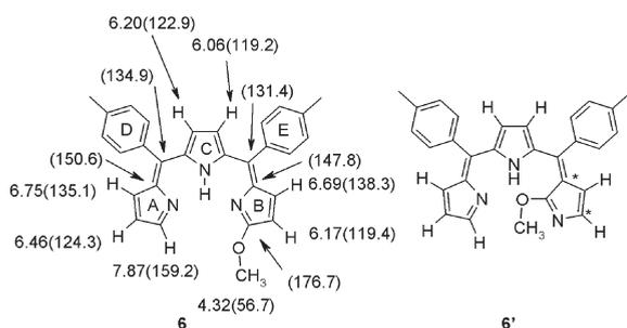
**FIGURE 1.**  $^1\text{H}$  and  $^{13}\text{C}$  NMR chemical shifts of **6** ( $\text{CDCl}_3$  solution) as well as an alternative structure **6'** (atoms marked by asterisks in the figure—see the explanation in the text).
