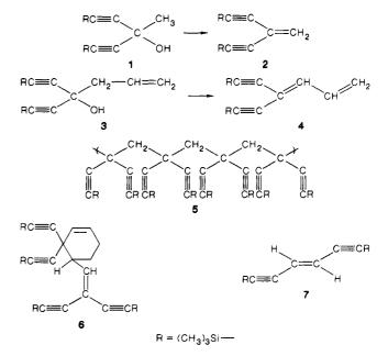
from addition of a 10-fold excess of allylmagnesium bromide to 1,5-bis((trimethylsilyl)ethynyl) ketone in dry ether at ambient temperature; 3 was purified by molecular distillation at 0.3 mm (bath temperature 85 °C) and obtained as a colorless oil. Dehydration analogous to the procedure for 2 gave 4 in 60% yield as a colorless liquid after chromatography over silica gel with pentane.
