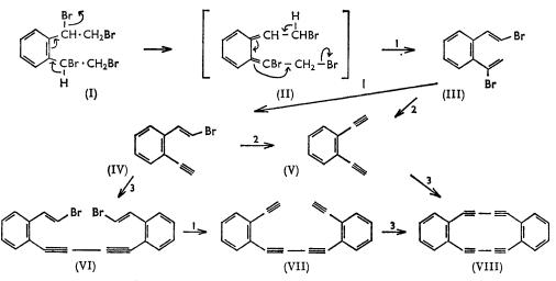
Reagents: I,  $Bu^{t}OK$  in  $Bu^{t}OH$ . 2,  $Bu^{t}OK$  in benzene. 3,  $Cu(OAc)_{2}$  in  $C_{5}H_{5}N$ -MeOH.
