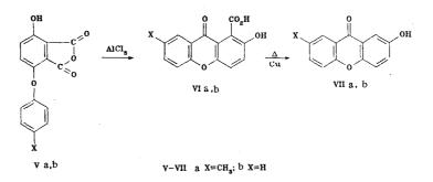
The compounds of type V underwent cyclization under the action of aluminum chloride and formed the hitherto undescribed 2-hydroxyxanthonecarboxylic acids of type VI with an 80-86% yield. The structure of the xanthonecarboxylic acids of type VI was confirmed by converting them upon decarboxylation into the known hydroxyxanthones of type VII [6, 7]. Hydroxyxanthone VIIa was also obtained by cyclization of an ester of 3-tolyloxy-6-hydroxyphthalic acid in polyphosphoric acid.
