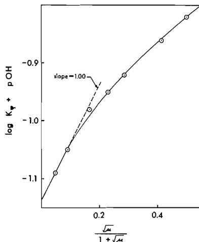
FIG. 1. A plot of  $\log k_b$  ( $\equiv \log k_{\psi} + \text{pOH}$ ) (in  $1 \text{ mol}^{-1} \text{ s}^{-1}$ ) against  $\sqrt{\mu}/(1 + \sqrt{\mu})$  for 1-acetyl-5,5-dimethyl-2-thiohydantoin at 25.4 °C.
