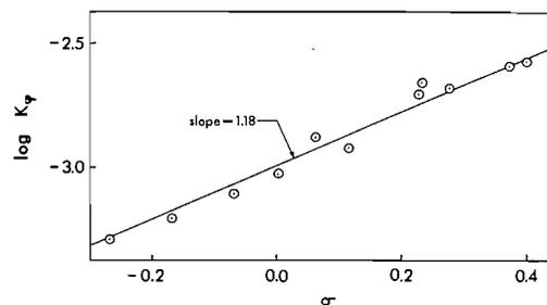
FIG. 5. A plot of  $\log k_{\psi}$  against  $\sigma$  for *m*- and *p*-substituted 1-benzoyl-2-thiohydantoin (c.c.: 0.9902; s.d.: 0.05) in aqueous phosphate buffer, pH 10.75,  $\mu = 0.42$ , at 25.3 °C.
