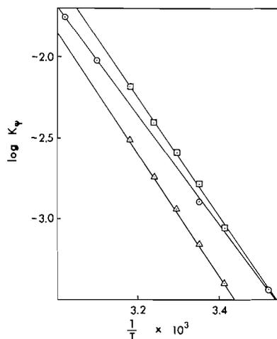
FIG. 2. Arrhenius plots for the hydrolysis of 1-acetyl-5,5-dimethyl-2-thiohydantoin (O), 1-benzoyl-2-thiohydantoin (□), and 1-acetyl-2-thiohydantoin (Δ) in phosphate buffer (see Table 5).
