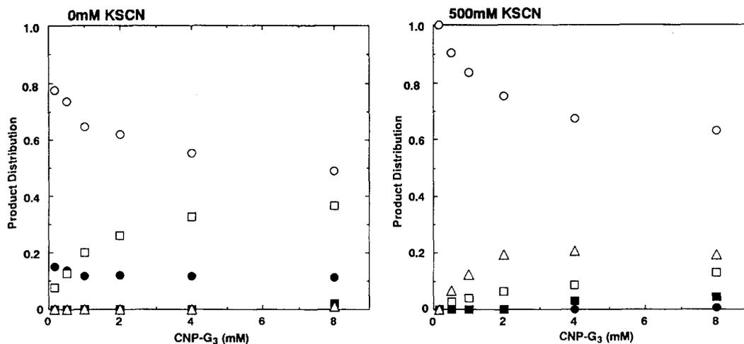
Fig. 4. The effect of the substrate concentration of CNP- $G_3$  on the product distribution of CNP-derivatives in the absence (left) and in the presence of 500 mM KSCN (right). The product distribution was calculated by a CNP-derivative (mol) divided by the sum of the CNP-derivatives (mol) in the products:  $\circ$ , CNP;  $\bullet$ , CNP- $G$ ;  $\square$ , CNP- $G_2$ ;  $\blacksquare$ , CNP- $G_4$ ;  $\triangle$ , CNP- $G_6$ .
