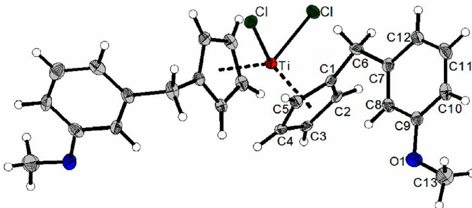
Fig. 7. X-ray diffraction structure of bis-[(3-methoxy-benzyl)cyclopentadienyl]titanium(IV) dichloride **3b** (thermal ellipsoids are drawn on the 50% probability level).
