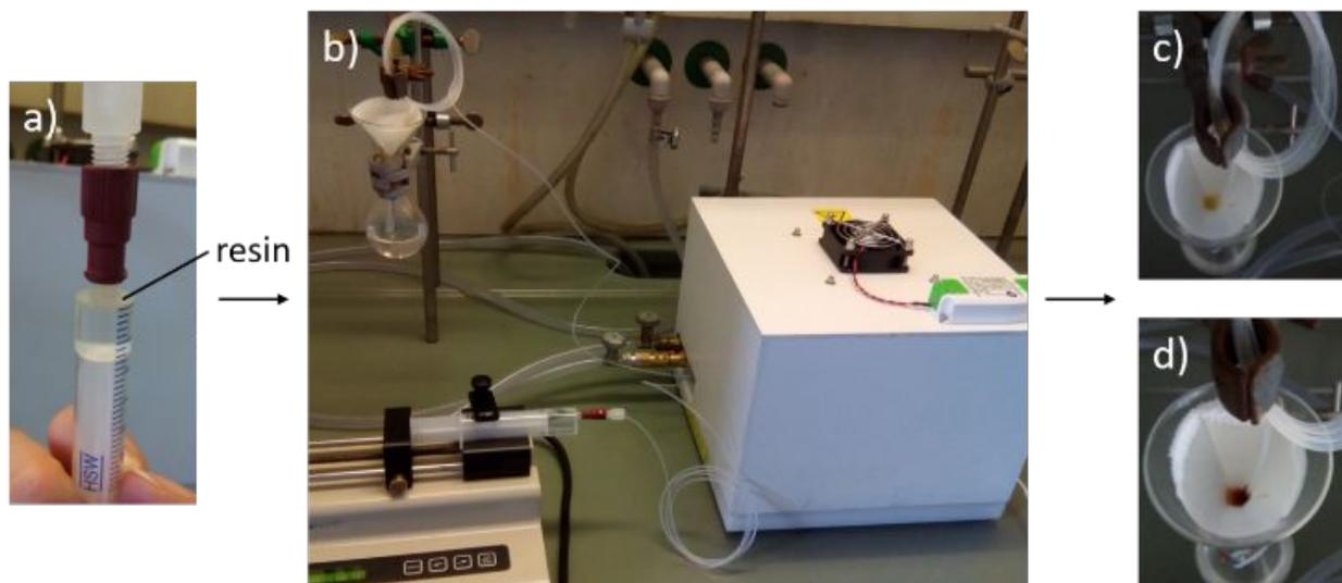
48 **Figure 3.** Workflow of the continuous flow photocleavage from solid support. a) Injection of the
