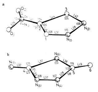
Fig. 1. Bond lengths and bond angles in 4-nitropyrazole (a) and 3-methyl-5-amino-1,2,4-triazole (b); the errors in the determination of the bond lengths and bond angles were 0.02-0.03 Å and 2-3°, respectively.
