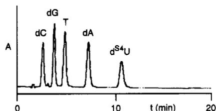
**Figure 1.** HPLC of enzymatic digestion of d(GACTCT<sup>S4</sup>UTT GAC) (**3**) into constituent deoxyribonucleosides. Detector at 254 nm initially and then 332 nm at 9 min. Ratio of dC/dG/T/dA/d<sup>S4</sup>U (3/2/4/2/1) was measured as 3.3:2.0:4.1:1.9:1.0.
