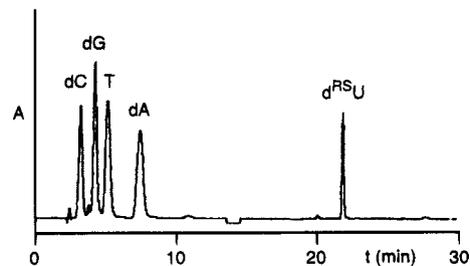
**Figure 3.** HPLC of enzymatic digestion of d(GACTCT<sup>RS4</sup>UTT GAC) (R = SCH<sub>2</sub>CH<sub>2</sub>CH<sub>2</sub>Cl, **16**). Detector at 254 nm, 332 nm at 9 min, and 308 nm at 14 min. Ratio of dC/dG/T/dA/d<sup>RS4</sup>U (3/2/4/2/1) was measured as 3.2:2.0:3.9:1.9:1.1.
