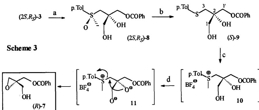
**Reagents and conditions:** a)  $\text{H}_2\text{O}/\text{HClO}_4/\text{THF}$ , r.t.; b)  $\text{NaI}$ ,  $(\text{CF}_3\text{CO})_2\text{O}$ ,  $\text{CH}_3\text{COCH}_3$ ,  $-40^\circ\text{C}$ ; c)  $(\text{CH}_3)_3\text{OBF}_4$ ,  $\text{CH}_2\text{Cl}_2/\text{CH}_3\text{NO}_2$ ; d)  $\text{LiH}$ ,  $\text{DMF}$ .
