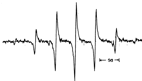
Fig. 3. ESR spectrum of trineopentylgermyl radical at -60^{\circ}\text{C} .
