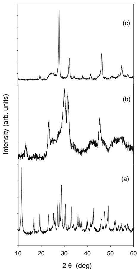
Fig. 1. XRD diffraction patterns of the sample prepared under solvothermal conditions ( $T = 160 \text{ }^\circ\text{C}$ ,  $t = 4 \text{ h}$ ) using ethanol as solvent and neodymium nitrate as starting material: (a) as-prepared, (b) heated at 500 °C, (c) heated at 800 °C.
