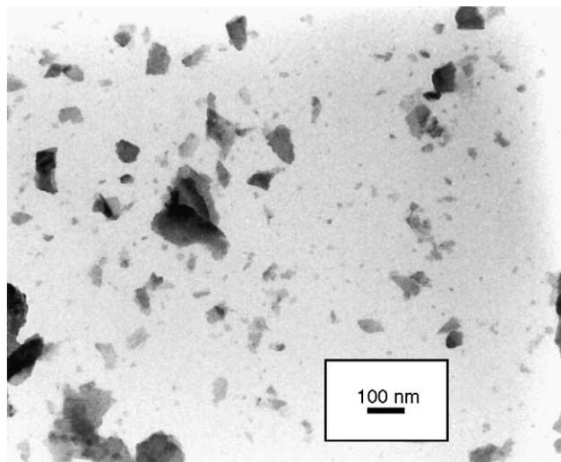
Fig. 2. TEM image of solvothermally prepared nanoparticles at 160 °C for 4 h using ethanol as solvent and neodymium nitrate as raw material.
