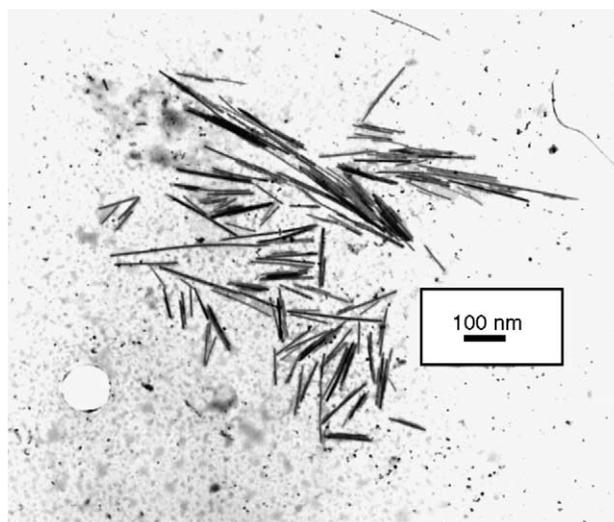
Fig. 6. TEM image of hydrothermally prepared needle-like nanoparticles at 160 °C for 4 h using neodymium acetate as precursor.
