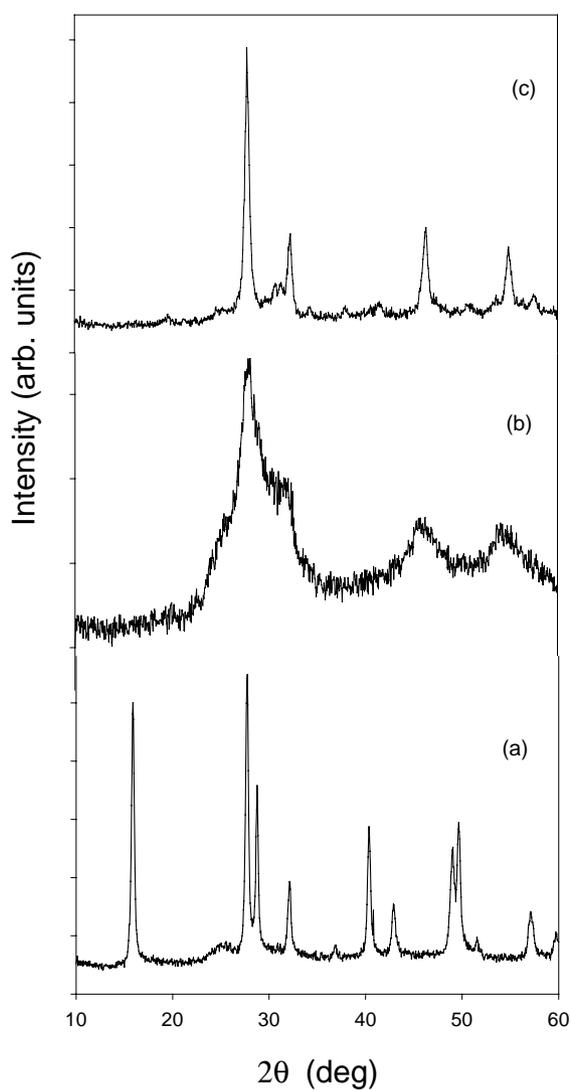
Fig. 5. XRD patterns of the sample synthesized under hydrothermal conditions ( $T = 160\text{ }^{\circ}\text{C}$ ,  $t = 4\text{ h}$ ) using neodymium acetate as starting material: (a) as-prepared, (b) heated at 500 °C, (c) heated at 800 °C.
