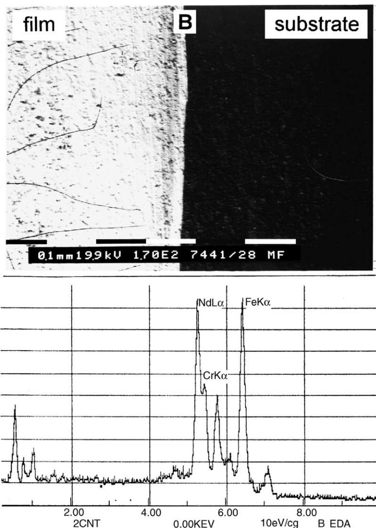
Fig. 8. SEM image of neodymium oxide thin film deposited on stainless steel substrate (prepared from fibrous precursor) and heated at  $1100^\circ\text{C}$ . EDS analysis confirmed the presence of  $\text{Nd}_2\text{O}_3$  film.
