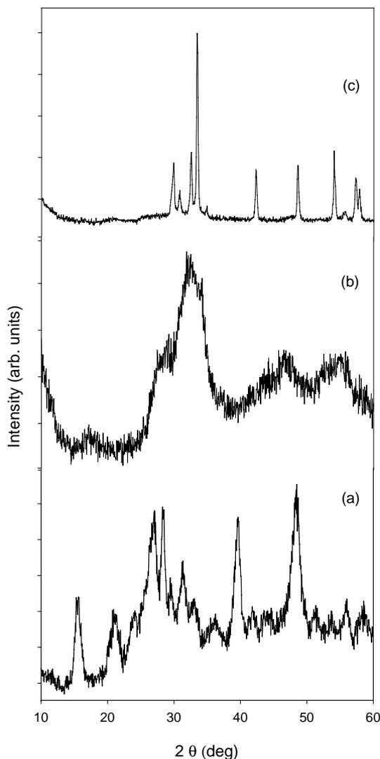
Fig. 3. XRD patterns of the sample synthesized under hydrothermal conditions ( $T = 140 \text{ }^\circ\text{C}$ ,  $t = 4 \text{ h}$ ) using neodymium acetate as starting material: (a) as-prepared, (b) heated at 500 °C, (c) heated at 800 °C.
