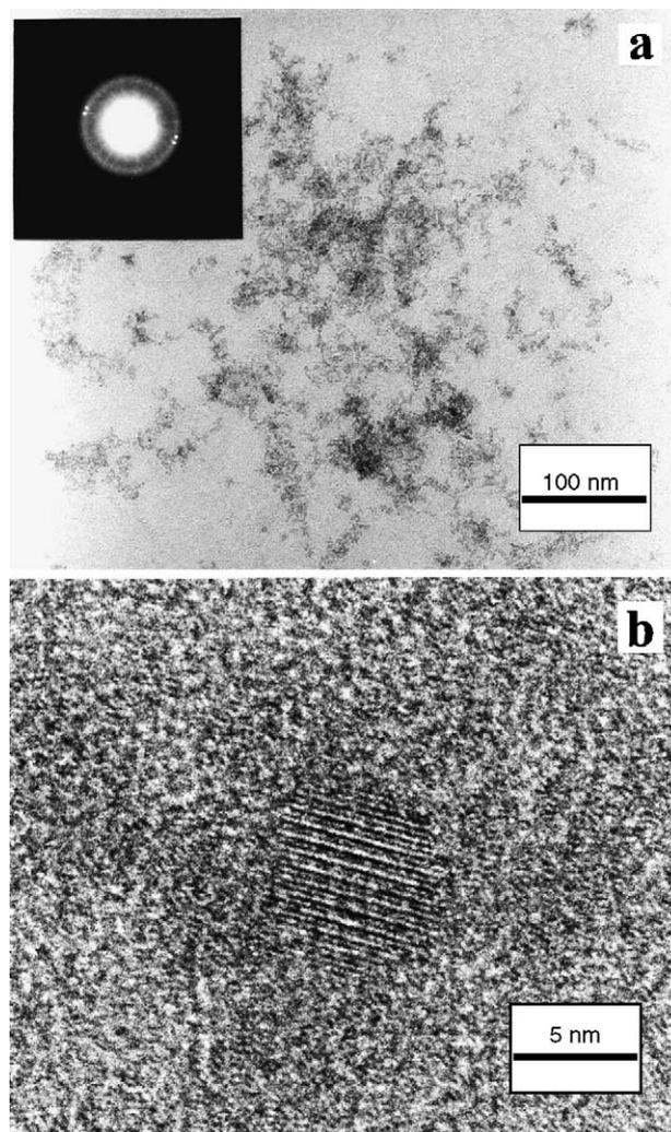
Fig. 7. TEM images of hydrothermally prepared spheroidal nanoparticles at 180 °C for 8 h using neodymium acetate as precursor ((a) low and (b) high magnification) with SAED pattern showing rings that match  $d$ -spacings for the structure of C-type neodymium oxide.
