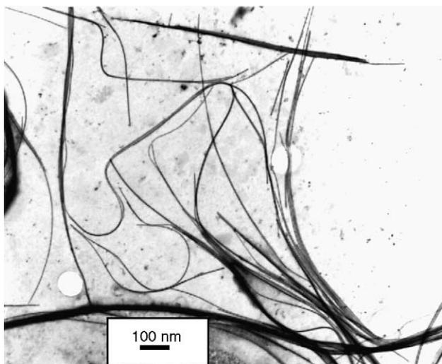
Fig. 4. TEM image of hydrothermally prepared fibrous nanoparticles at 140 °C for 4 h using neodymium acetate as precursor.
