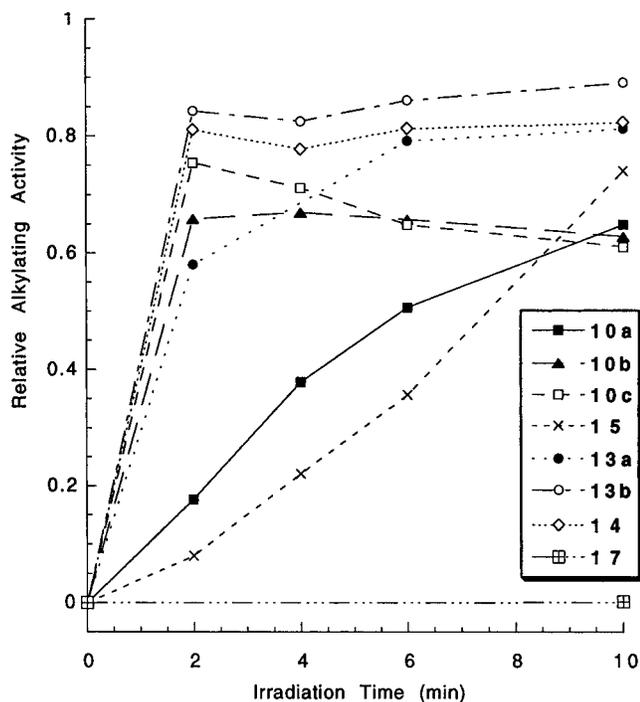
**Figure 3.** 4-(4-Nitrobenzyl)pyridine (NBP) assay of irradiated solutions ( $t = 0, 2, 4, 6, 10$  min) of **10a–c** and **15** (in  $\text{CH}_3\text{CN}$ ), **13a,b** and **14** (in  $\text{H}_2\text{O}$ ), and **17** (in  $\text{EtOH}/\text{H}_2\text{O}$  1:1). The relative alkylating activity was determined by measuring the absorbance of the alkylated NBP chromophore at  $\lambda = 542$  nm. The numbers are relative numbers. See the text and Experimental Section for details.
