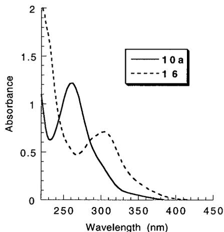
**Figure 1.** UV spectral recording of the photolysis of nitrobenzylphosphoramidate mustard (**10a**) in acetonitrile solution (0.2 mmol). The sample was photolyzed in a quartz cuvette (1 cm path length) for 20 s to give **16** ( $\lambda_{\text{max}} = 304$  nm).
