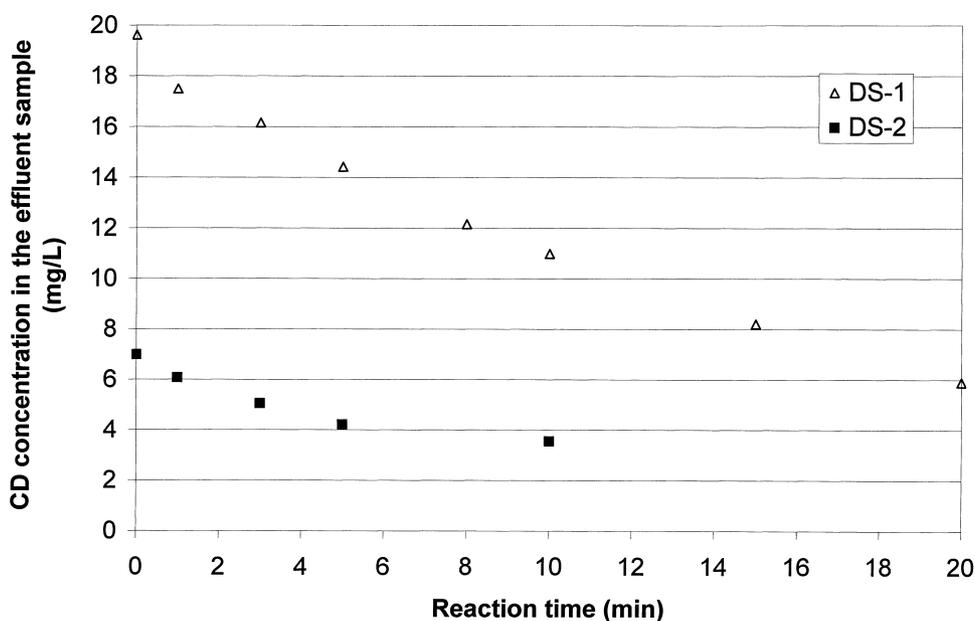
Fig. 6. The reduction in the CD concentration of the effluent samples DS-1 and DS-2 as a function of ozonation time.
