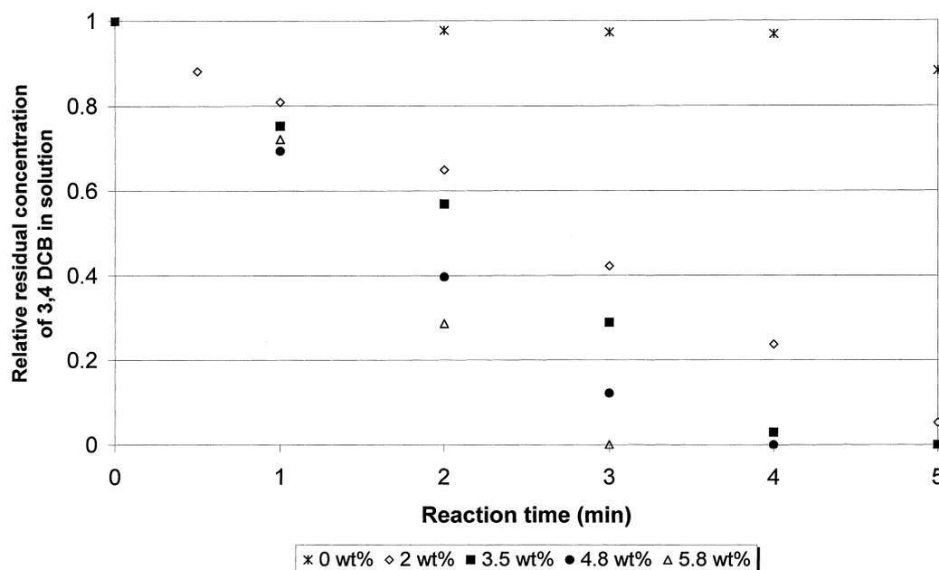
Fig. 2. The effect of ozone concentration on the oxidation rate of 3,4 DCB in solutions with initial concentration of 20 mg/l.
