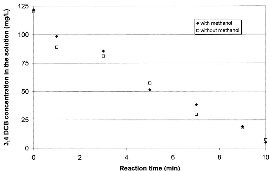
Fig. 3. The effect of methanol on the ozone oxidation rate.
