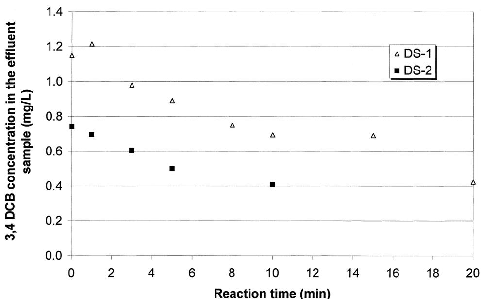
Fig. 5. The reduction in the 3,4 DCB concentration in the effluent samples DS-1 and DS-2 as a function of ozonation time.
