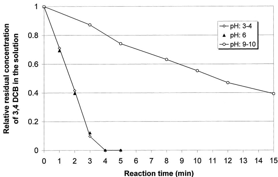
Fig. 4. The influence of pH on the oxidation rate of 3,4 DCB in the solutions with initial concentration of 20 mg/l.
