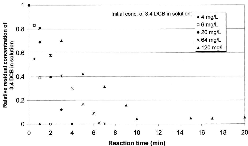
Fig. 1. The effect of initial concentration of 3,4 DCB on the oxidation rate at an ozone concentration of 4.8 wt%.
