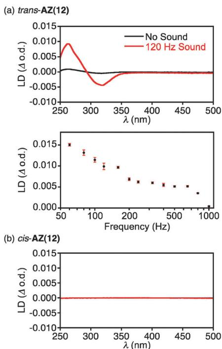
Fig. 4 LD spectra of (a) *trans*-AZ(12) and (b) *cis*-AZ(12) in cyclohexane ( $4.0 \times 10^{-5}$  M) at 20 °C with and without 120 Hz sound irradiation (red and black curves, respectively). Changes in LD intensity of (a) at 261 nm by varying sound frequencies with the amplitude of 13.5 Pa. The obtained LD intensities were averaged for 50 s.
