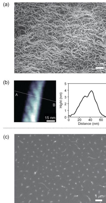
Fig. 3 Scanning electron micrographs of air-dried samples of (a) *trans*-AZ(12) and (c) *cis*-AZ(12) prepared from a cyclohexane solution with a concentration of  $4.0 \times 10^{-5}$  M deposited on a specimen grid covered with a thin carbon support film. (b) FM-AFM image and height profile (positions A to B) of a *trans*-AZ(12) fiber on the HOPG surface immersed in pure water. Cantilever oscillation amplitude: 0.2 nm. Frequency-shift setpoint: +80 Hz.
