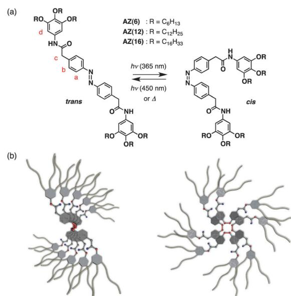
Fig. 1 (a) Chemical structures of *trans*-AZ(*n*) and *cis*-AZ(*n*) (*n* = 6, 12, and 16), and (b) their possible self-assemblies.
