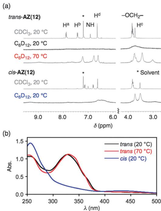
Fig. 2 (a) <sup>1</sup>H NMR spectra of *trans*-AZ(12) at 20 and 70 °C and *cis*-AZ(12) at 20 °C in CDCl<sub>3</sub> or cyclohexane-*d*<sub>12</sub> with a concentration of  $1.2 \times 10^{-2}$  M. (b) Absorption spectra of *trans*-AZ(12) at 20 and 70 °C and *cis*-AZ(12) in cyclohexane with a concentration of  $4.0 \times 10^{-5}$  M.
