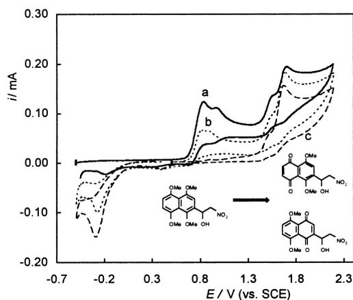
Figure 1. Cyclic voltammograms for the 2-(1-hydroxy-2-nitroethyl)-1,4,5,8-tetramethoxynaphthalene (on Pt, at  $0.2 \text{ V s}^{-1}$ ) performed before and after the electrolysis carried out at the first oxidation step. (a) Starting reaction mixture; (b) after 1 faraday/mole at 0.9 V; (c) after 2 faraday/mole at 0.9 V
