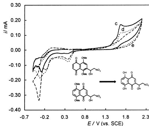
Figure 2. Cyclic voltammograms for the 2-(1-hydroxy-2-nitroethyl)-1,4,5,8-tetramethoxynaphthalene performed before and after the electrolysis carried out at the second oxidation step. (c) Reaction mixture at the end of the oxidation at 0.9 V; (d) after 0.6 faraday/mole at 1.7 V; (e) after 3.0 faraday/mole at 1.7 V
