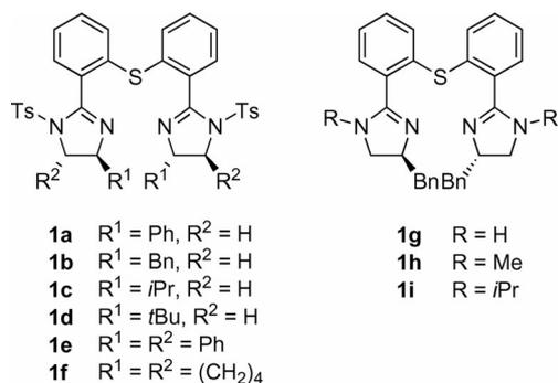
Figure 1. Diphenyl sulfide linked bis(imidazoline) ligands.
