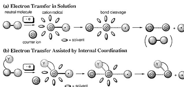
neutral molecule. In this paper we describe experimental and theoretical studies of intramolecular assistance by dynamic coordination of carbonyl groups and heteroatoms to tin in the electron transfer driven reaction of tetraalkylstannanes.
