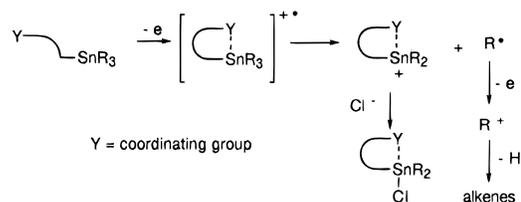
lecular coordination. Such stabilization favors the electron transfer to decrease the oxidation potential. It is also noteworthy that in **A** and **B** one of the carbon-tin bonds is selectively elongated. Therefore, the intramolecular coordination is also responsible for the selective cleavage of the C-Sn bond.
