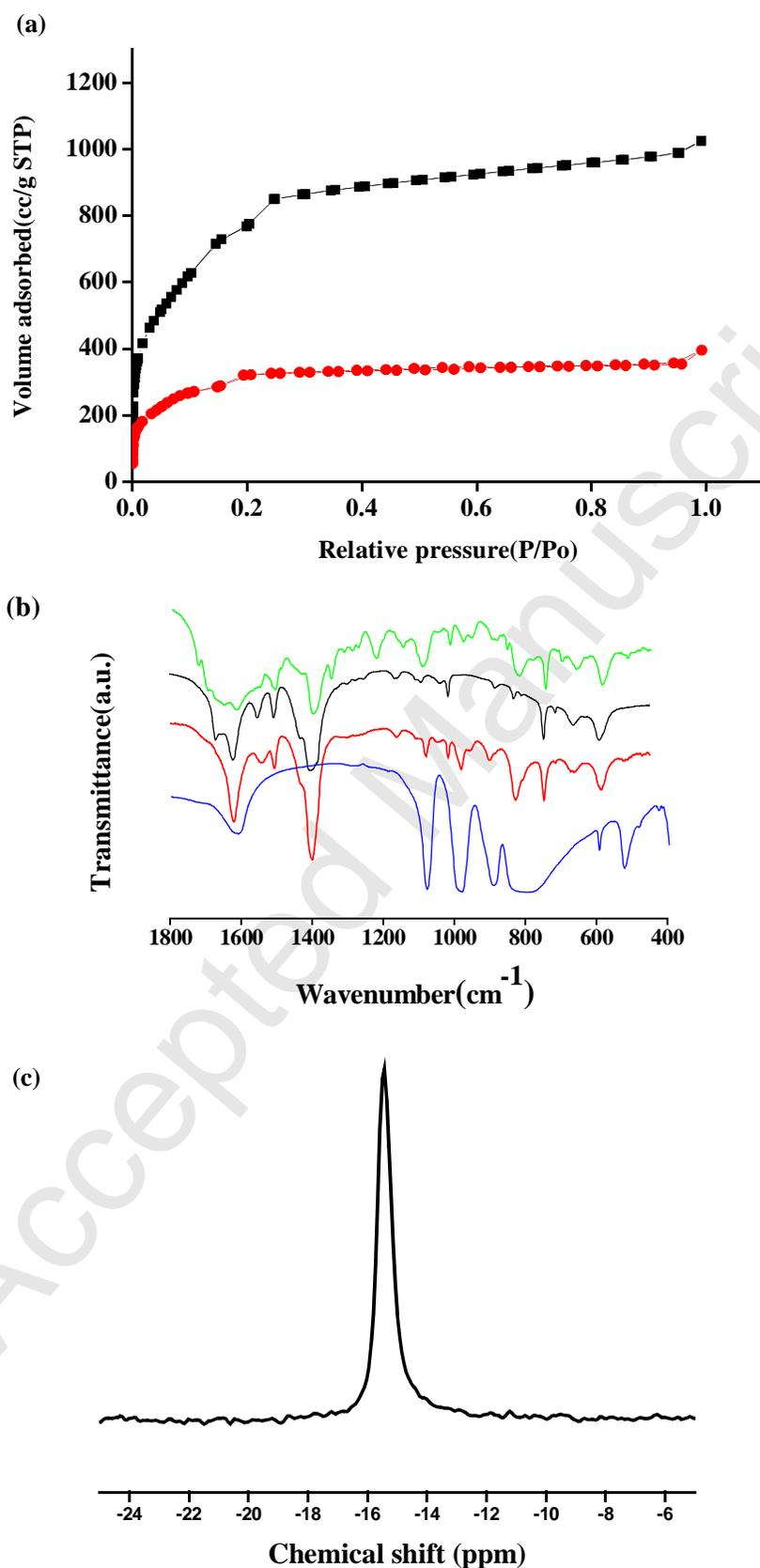
Fig. 3 (a) N<sub>2</sub> adsorption isotherm of MIL-101(Black), PTA@MIL-101(red), (b) FT-IR spectra of recovered PTA@MIL-101(Green), MIL-101(Black), PTA@MIL-101(red) and PTA(blue) (c) <sup>31</sup>P solid state MAS NMR spectrum of PTA@MIL-101
