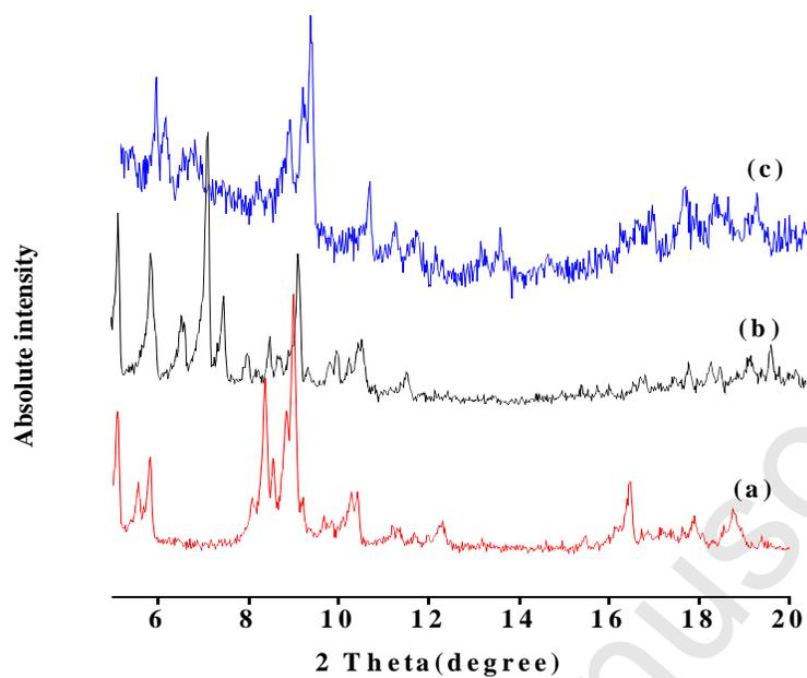
Fig.1 PXRD pattern of (a) MIL-101, (b) PTA@MIL-101, (c) recovered PTA@MIL-101
