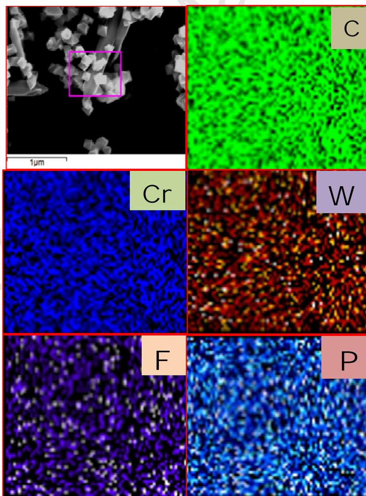
Fig.2 EDS mapping images of different elements of PTA@MIL-101
