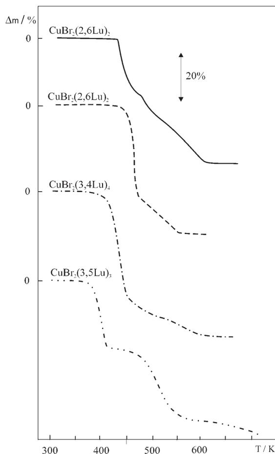
Fig. 4 TG curves for the copper(II) bromide complexes with lutidines
