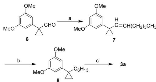
**Scheme 2.** Reagents and conditions: (a) Br<sup>−</sup> Ph<sub>3</sub>P<sup>+</sup>-(CH<sub>2</sub>)<sub>4</sub>CH<sub>3</sub>, (Me<sub>3</sub>Si)<sub>2</sub>N<sup>−</sup>K<sup>+</sup>, THF, rt, 2 h, 96%; (b) TsNHNH<sub>2</sub>, CH<sub>3</sub>COONa, DME, H<sub>2</sub>O, reflux, 5 h, 96%; (c) 9-*I*-9-BBN, hexane, −78 °C to 0 °C, 3 h, 95%.
