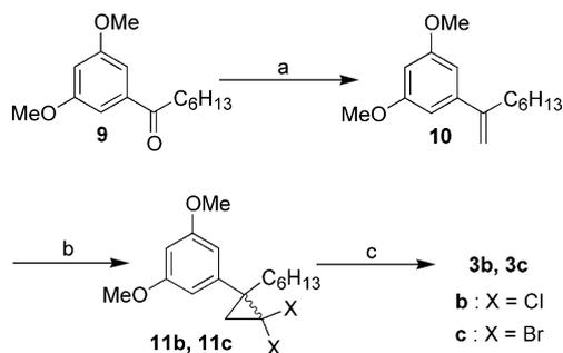
**Scheme 3.** Reagents and conditions: (a) I<sup>−</sup> Ph<sub>3</sub>P<sup>+</sup>-CH<sub>3</sub>, (Me<sub>3</sub>Si)<sub>2</sub>N<sup>−</sup>K<sup>+</sup>, THF, rt, 1.5 h, 93%; (b) Me<sub>3</sub>CO<sup>−</sup>K<sup>+</sup>, CHX<sub>3</sub>, hexane, −10 °C to rt, 2–2.5 h, 56–89%; (c) BBr<sub>3</sub>, CH<sub>2</sub>Cl<sub>2</sub>, −78 °C to −20 °C, 3 days, 63–86%.
